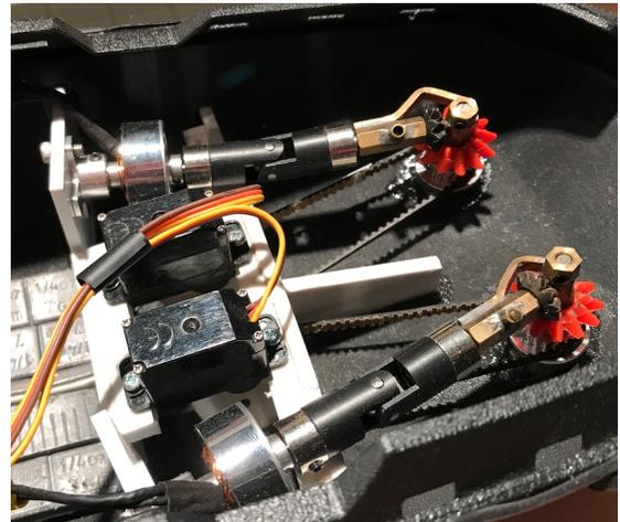
Above left is the tug with the basic pieces in place-- Eric is working on the detailing. The photo on the right shows the drivetrain. You can see the two brushless motors with their universal joints that send the power to the prop via the bevel gears. Between the two motors are a pair of steering servos, mounted upside down. The servos have pulleys instead of arms, and you can see the toothed drive belts that rotate the drive units.
