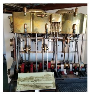
Charlie sent this photo a triple-expansion steam engine from 1916. It powered JP Morgan's commuter yacht Navette. By this time, internal combustion engines had generally replaced steam but Morgan preferred the much quieter steam plant over a noisy gas engine. Steam was very expensive luxury, as it needed a larger boat to allow for the extra space it needed, plus you needed licensed Steam Engineers to operate it.
