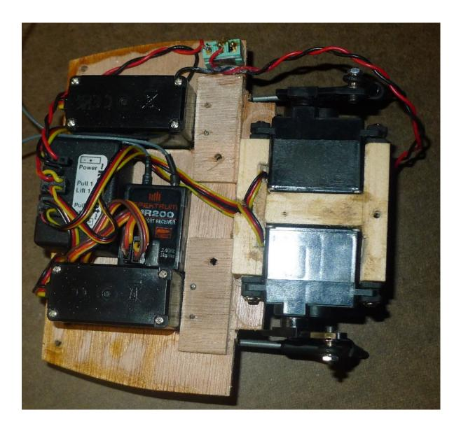
In the above view, between the pull servos sits the microcontroller and the Spektrum MR200 receiver. Given the need to make the installation compact all the leads were trimmed to the shortest possible.
