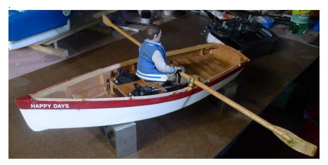
The boat hull is 12" long, made from a Bevin's Skiff Scale Model kit from Chesapeake Light Craft. The sheers were raised by about 1/4" to provide enough depth for the servos to sit appropriately.
