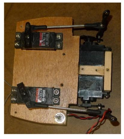
In the view to the right, two pull servos on the left are standard size HS-485BB's. On the right are the two lift servos, the more compact HS82MG.
