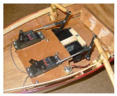
A central platform provides the mounting of the servos, the receiver, and the microcontroller.
